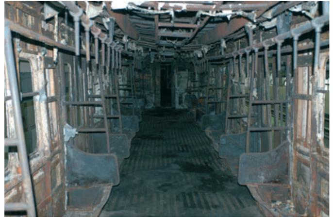
FIG. 5—An interior structure of the room of the number 1080 train after the recovery when nothing was left except for the steel frame of the train.
