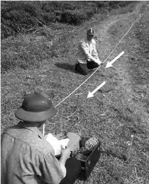
Figure 13.7 Soil-resistivity testing can be accomplished with minimal equipment. A resistivity survey of a site in Vietnam illustrates readings being taken along transects with the electrodes (arrows) spaced at 2-meter intervals.
