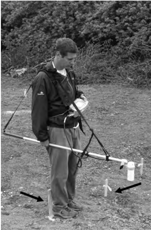
Figure 13.8 Cesium magnetometers are portable and readily usable by single investigators. Note that the readings are being taken at 1-meter intervals marked by wooden stakes.
