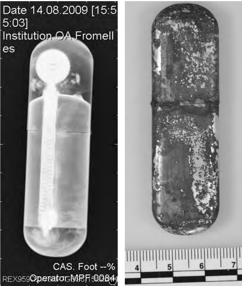
Figure 39.3 Radiograph of a heavily corroded cigarette lighter
