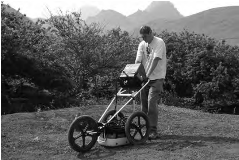
Figure 13.10 Ground-penetrating radar equipment is increasingly becoming more portable. Many of the devices now are cart-mounted and can be used with minimal ground-surface preparation.
