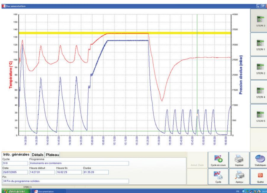
Figure 12 Vacuum pump graph
